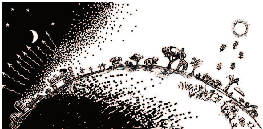
Fig. 2.9 Photons arriving at the Earth's surface from the Sun have higher energy (shorter wavelength) than those returned to space by the Earth. Given an overall energy balance (the Earth does not get hotter over time), there must be more photons leaving than arriving; that is, the energy arriving has lower entropy than that departing.
